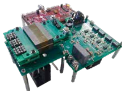
Power transformer for electrical converter (ENERSYS collaboration)
