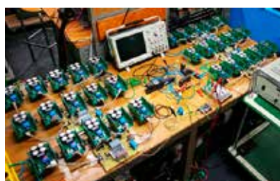
Design and realization of a three-phase full bridge MMC converter with 6 levels
